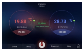
Real-time display of temperature change rate and steady state
